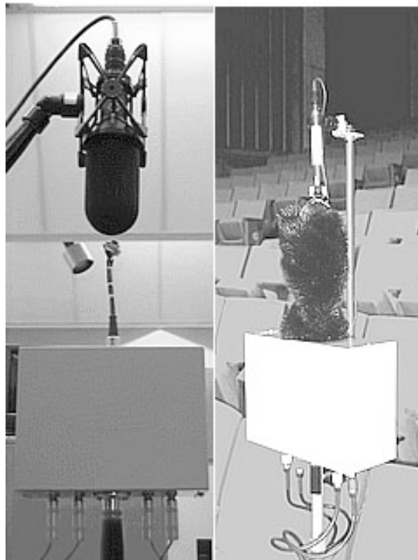
Figure 5 – Soundfield SPS422B and experimental mic without its windscreen (left). Experimental mic with windscreen and Core Sound TetraMic on the dual mount (right).
