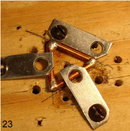
21-24. Reset the metal brackets to be clamps rather than guides for the triangle.
