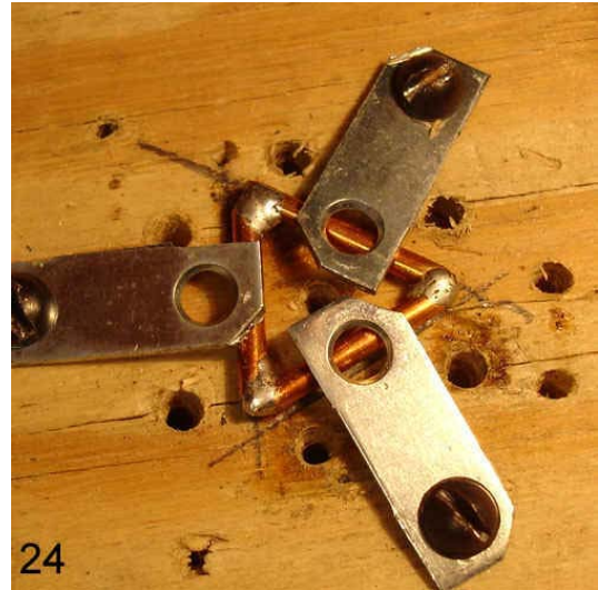
21-24. Reset the metal brackets to be clamps rather than guides for the triangle.
