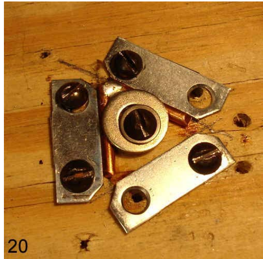
19-20. Turn it over and resolder. Let it cool and remove the uni-angle.
