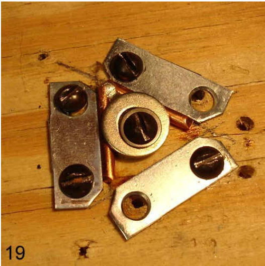
19-20. Turn it over and resolder. Let it cool and remove the uni-angle.
