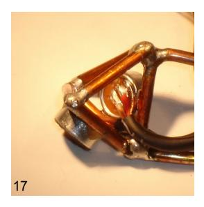
17. Capsule 2. Note the final routing of wire pair 2. Capsule 2 is the RFD (right-front-down) capsule.
