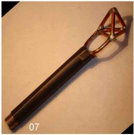
06-07. Slide a 2 <sup>3</sup>/<sub>4</sub>-inch piece of shrinkable tubing over the all-thread of the tetrahedral frame. It should leave about <sup>1</sup>/<sub>4</sub>-inch of thread at the bottom and cover the soldered junction of the pipe to the U-frame.
