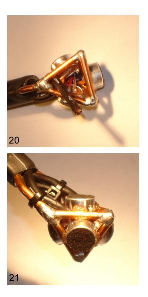
20. There is not much space for pair 4. Be sure the epoxy for the first 3 capsules is well set before continuing to the final capsule. Note the wire routing of the number 4 pair.
