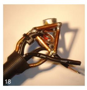
18. Capsule 2 in place with the epoxy set for a half hour. Before adding the tie-wrap, be certain the pairs lie next to the copper wire of the U-frame. If not, push more wire up from the bottom of the pipe. Pull the tie-wrap just snug.
