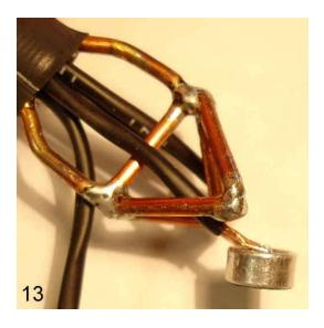
13. Gently pull the number 1 pair from the *bottom* of the pipe. If you need some capsule rotational alignment, twist the number 1 pair while pulling from the bottom; the capsule should follow the twist. If not, the 4 pairs of wires are probably not straight in the pipe. Straighten them (see step 8 above) and try again.
