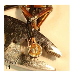
11. Route the pair through the tetrahedral as shown. Tie a rubber band around the handles of a pair of regular pliers so it will just hold a capsule securely. The pliers should be easy to open and close with just a little pressure. Place the capsule in the jaws as shown.
