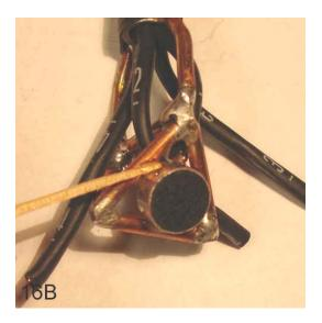
Grasp the tetrahedral and place your index finger or thumb on the face of the capsule. Carefully and accurately apply *slight* pressure to seat the capsule. Check that the capsule is centered and facing properly, flat to the face of the tetrahedral. Hold the capsule in this position for ONE HALF HOUR! DO NOT SHORTCUT THIS TIME! 16B. Roll the epoxy with the toothpick into the valley formed by the capsule and its supporting wire. Do this for all 3 edges.
