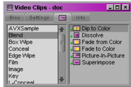
Blend effect category in the Effect Palette when real-time effects are enabled. Green dots indicate that the effects might preview in real time.
