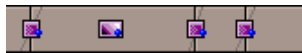
Effect icons in the Timeline when real-time effects are disabled. Blue dots indicate that the effects will not preview in real time.
