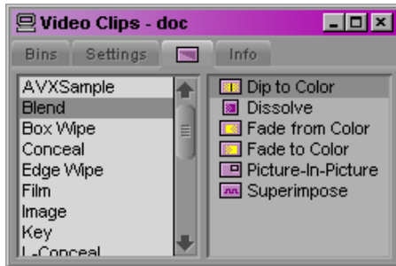
Blend effect category in the Effect Palette when real-time effects are disabled. No dots indicates that the effects will not preview in real time.
