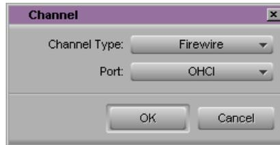
Channel refers to the signal path for deck control. If you have connected a DV camera or video deck that supports IEEE 1394, choose FireWire as the Channel Type and 1394 as the Port from the pop-up menus.
