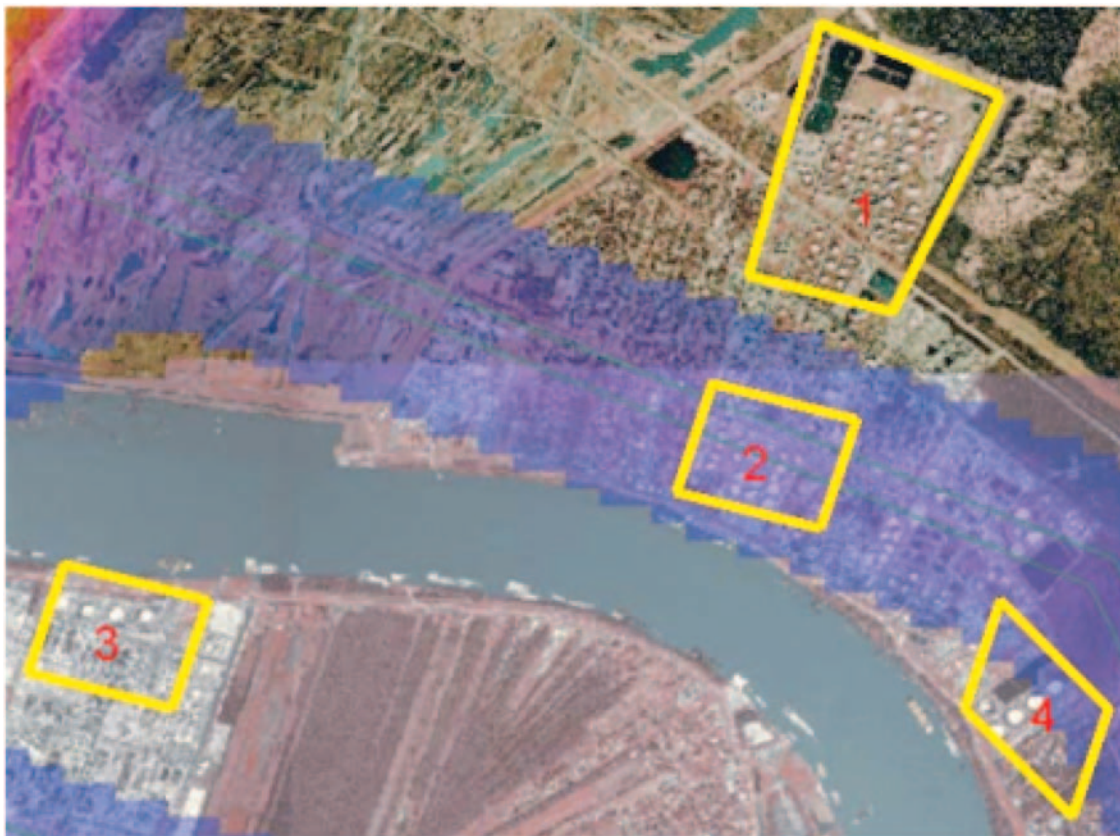
Figure 4. The yellow squares indicate facilities that have a high risk of power failures and the prioritization of diesel generator allocation to ensure a minimization of downtime and rapid recovery of key critical energy assets.
