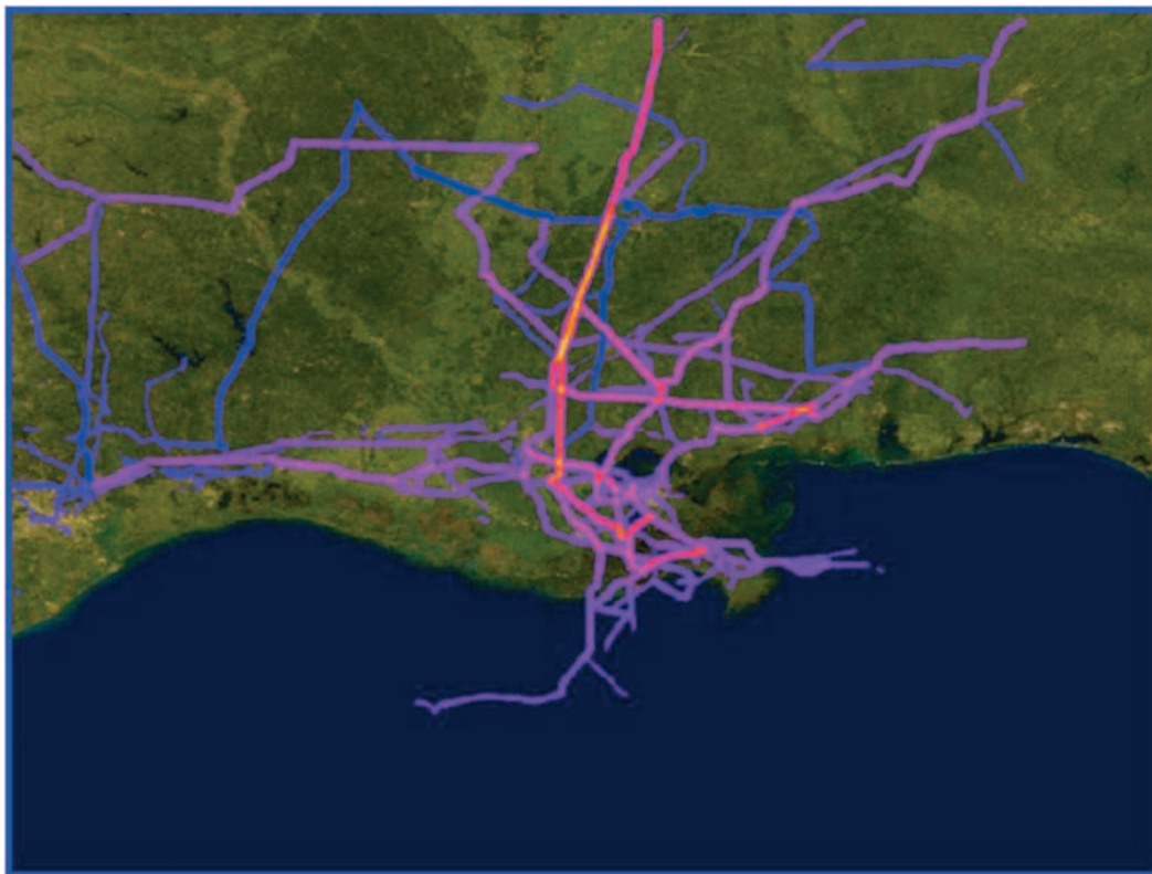
Figure 2. Interdependent analysis of energy infrastructure simulating the impact of the approaching hurricane. The areas fading from purple (low) to yellow (high) indicate areas that have lost connectivity because of predicted damage by the storm. The areas in blue have become congested and caused delays because of rerouting around failed infrastructure assets.
